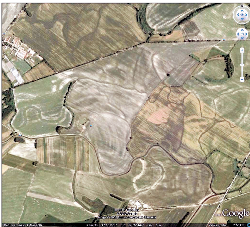
Fig. 2. Example of orthophoto map suitable for reconstruction of the original river network.
