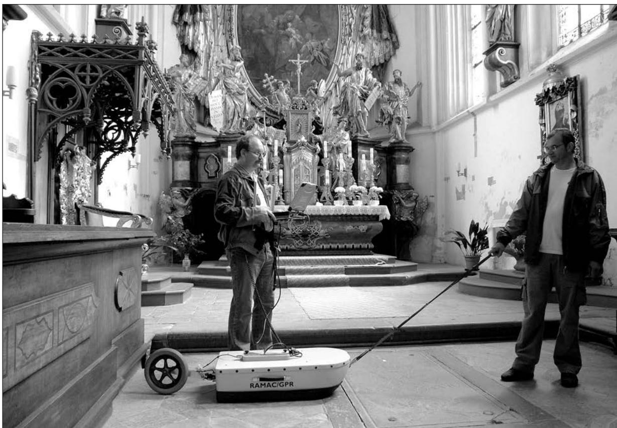
Photo 3. Radar measurement in the area of the presbytery of the conventual church of Birth of the Virgin.
