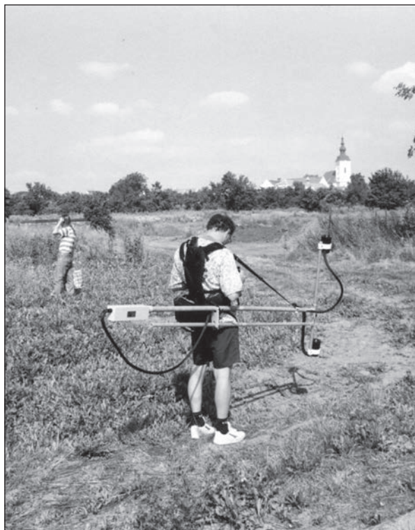
Photo 5. The GSMP-30 GEM SYSTEMS K-magnetometer (Canada) measurements. Photo by V. Hašek.
