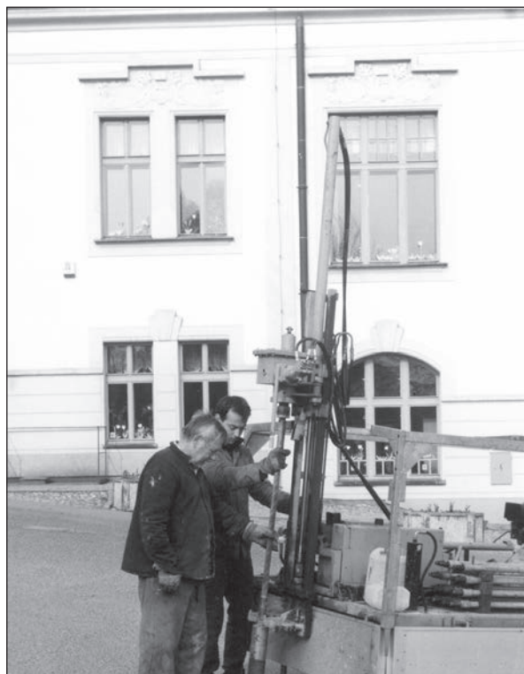
Photo 8. Pedological probing and verification of geophysical anomalies. Photo by V. Hašek.
