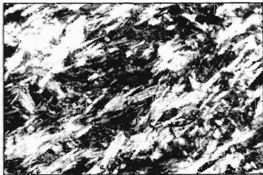
Fig. 3. Schistose pattern - nematoblastic texture of the actinolitic schist. Enlargement 90x, crossed polars.
